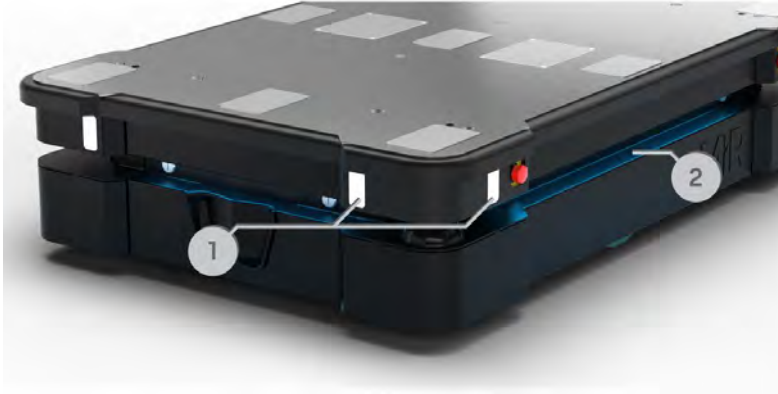
Figure 10.13. Indicator lights on MiR1350.
