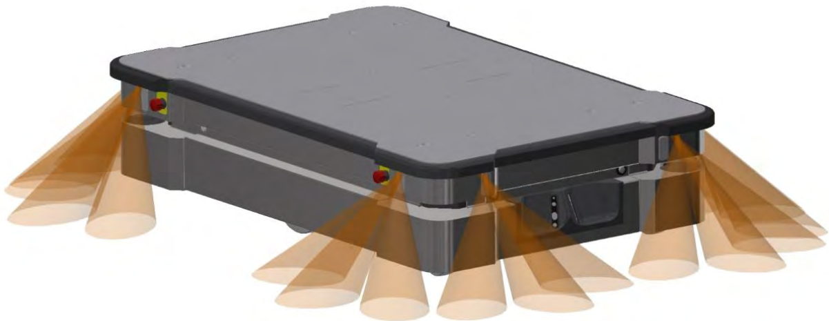
Figure 9.9. The proximity sensors in the corners of the robot detect objects below the safety laser scanners' plane of view.
