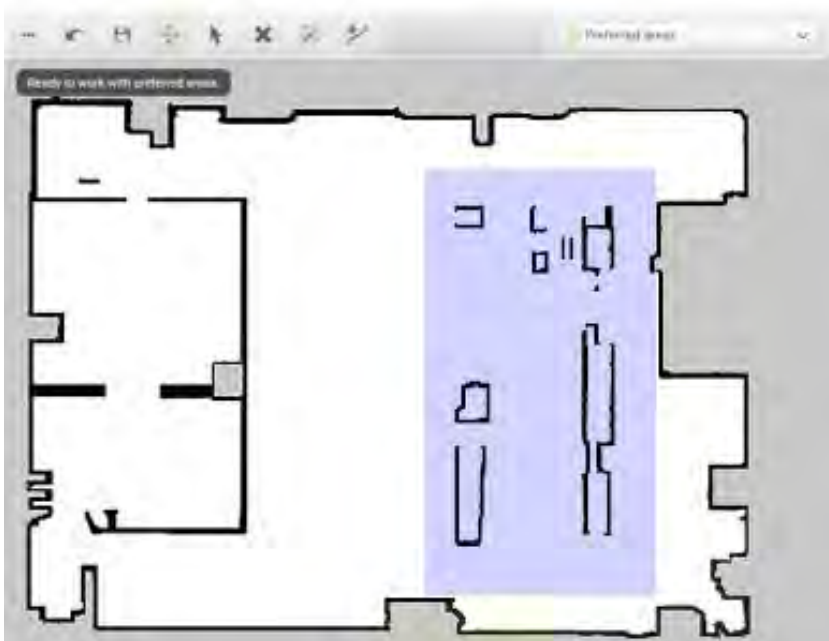
Figure 11.4. Unpreferred zones (marked with purple) can be used in highly dynamic areas to solve issues with replanning of paths.
