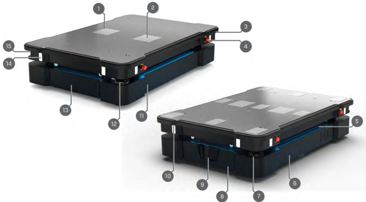
Figure 2.1. MiR1350 external parts.
