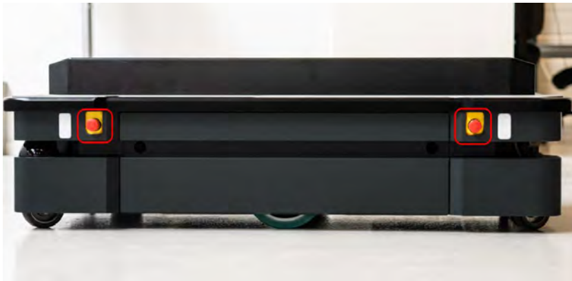
Figure 10.1. MiR1350 has four Emergency stop buttons and the option to connect additional Emergency stop buttons through the electrical interface.
