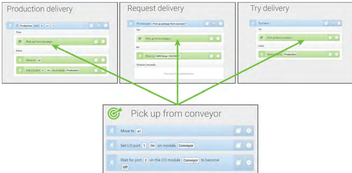
Figure 11.16. You can embed small missions into other missions. In this example, the mission Pick up from conveyor is used in three different missions. If you want to change how the robot picks up a package from the conveyor, you only need to change it once in the original mission instead of three times in each individual mission.
