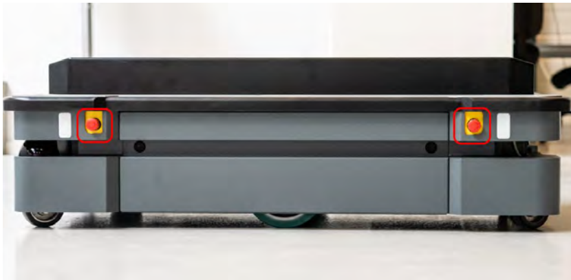
Figure 10.1. MiR600 has four Emergency stop buttons and the option to connect additional Emergency stop buttons through the electrical interface.
