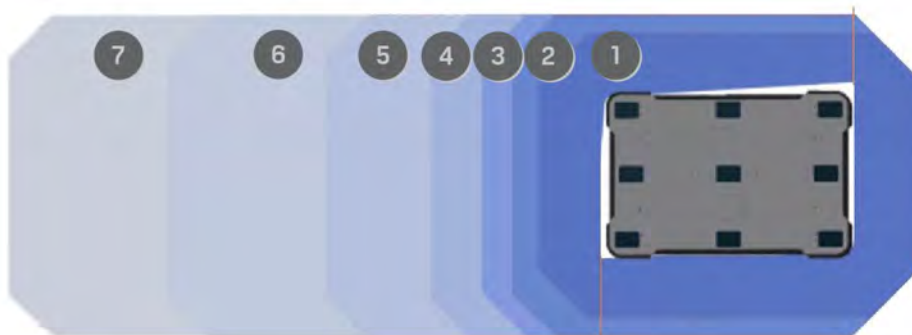
Figure 10.6. The illustration shows the field set contours when driving backward. The range of the active field changes with the robot's speed. The illustration also shows how the front scanner reduces its Protective field to a minimum when the robot moves backward.
