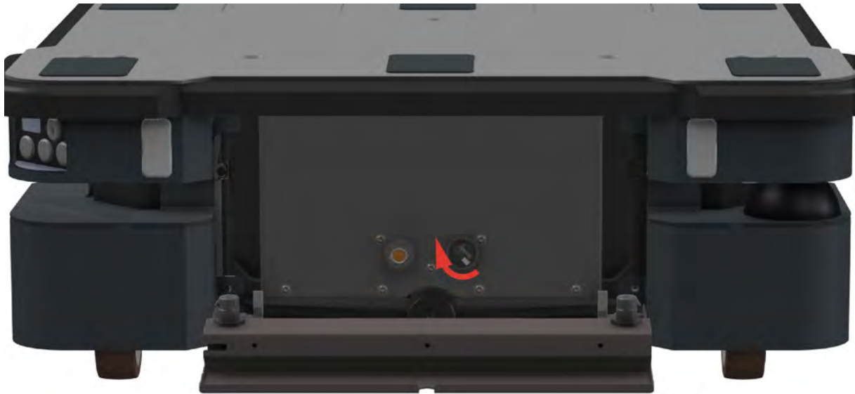
Figure 2.11. Turn the Manual brake release switch clockwise to release the brakes.
