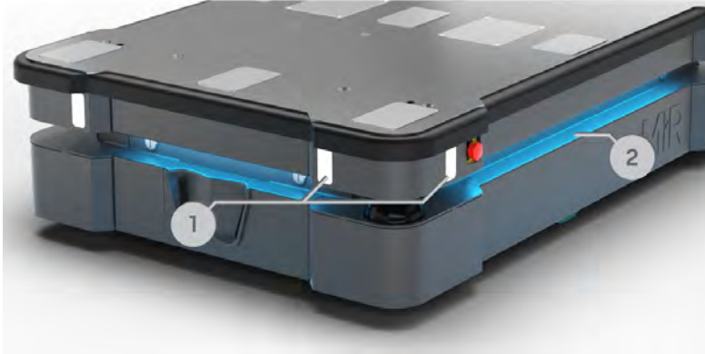
Figure 10.13. Indicator lights on MiR600.
