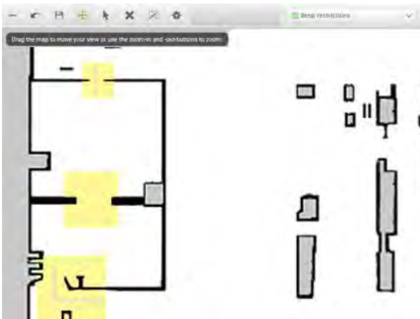
Figure 11.5. Narrow doorways can be marked with a Sound and light zone (marked with yellow) to warn people that a robot is coming through. A Critical zone (orange) can be placed in the narrow doorway to enable the global planner to make a path through the corridor.
