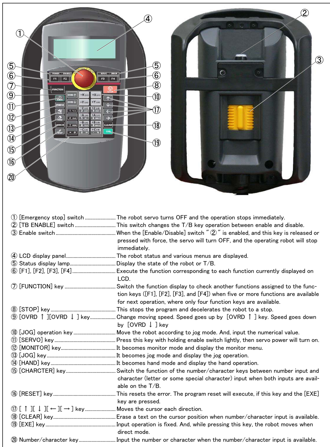
Fig.3-22 : Teaching pendant key layout and main functions
